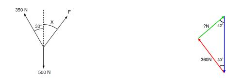
Solve by drawing a vector diagram to represent the forces. Represent the 500N vertical force with a 5cm vertical line. From the bottom of the line, add a 3.6cm line at  $30^{\circ}$ . Then join the two ends to form a triangle. The length and angle of the third line gives the third force (260N) and angle ( $42^{\circ}$ ).
