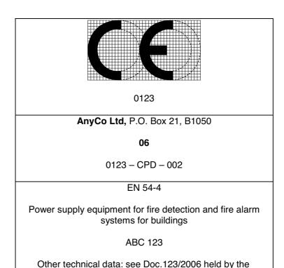
Figure ZA.1 — Example of CE marking information in the accompanying commercial documentation
